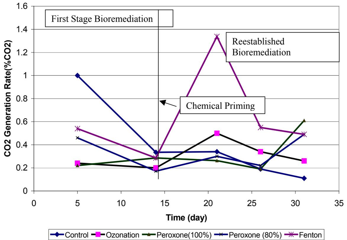
Figure 5.11. CO<sub>2</sub> Evolution from BIO/OX/BIO Treatment of the LMW-Soil
