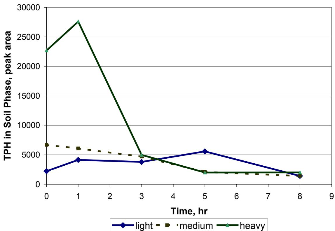
Figure 4.7. Results of Slurry Phase Fenton's Reagent Rate Test for the LMW-Soil
