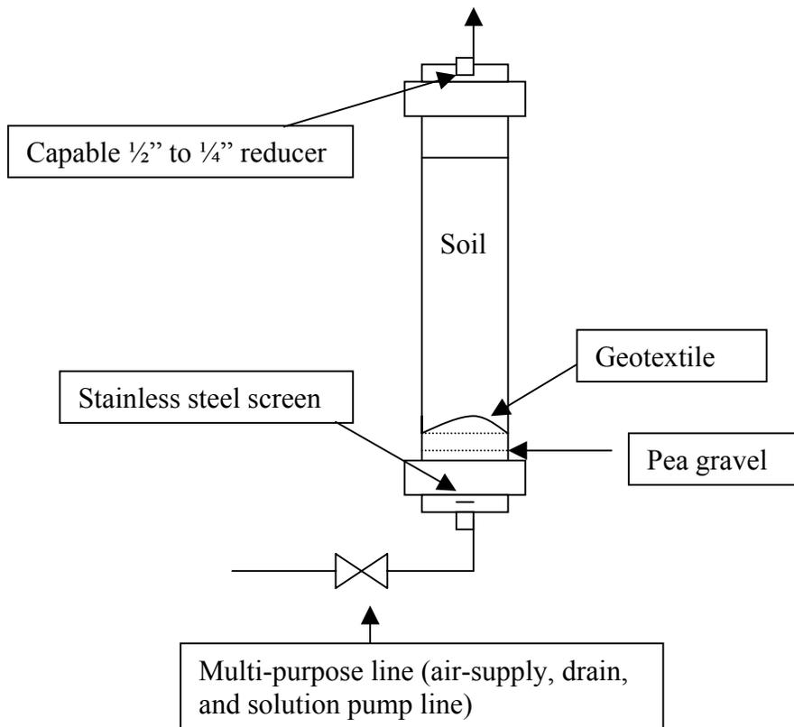
Figure 3.3. Schematic of a Bench Scale Column Reactor
