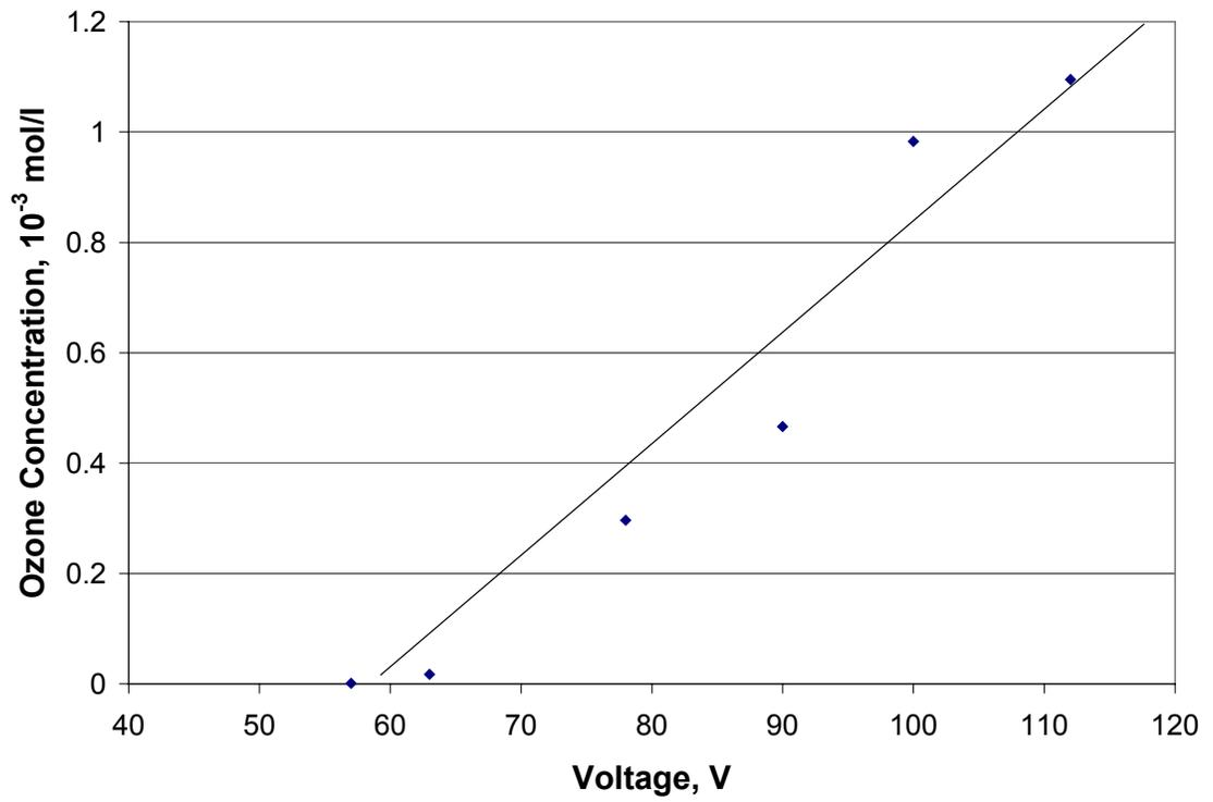
Figure 3.1. Ozone Concentration vs. Voltage (Flow Rate = 2 scfh)
