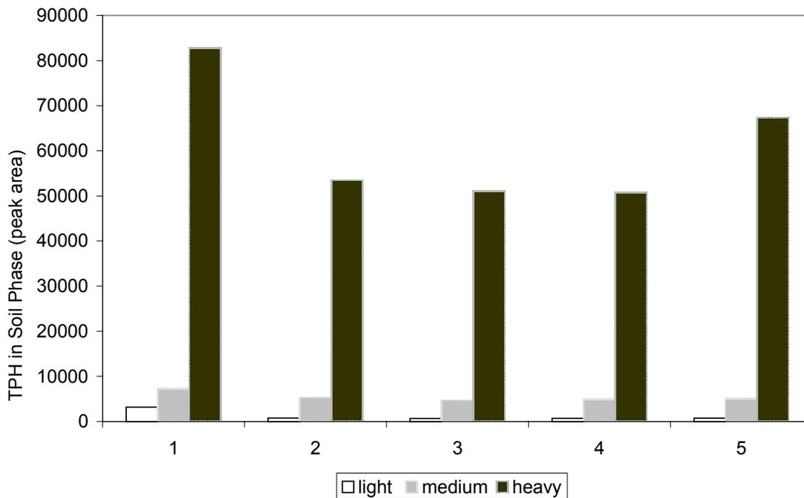
Figure 4.2. Soil Phase TPH Results of Slurry Phase Chemical Priming for the HMW-Soil
