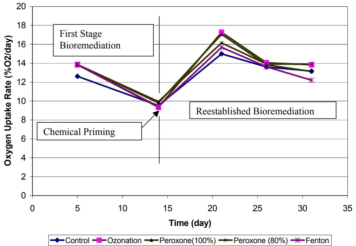
Figure 5.10. O<sub>2</sub> Evolution from BIO/OX/BIO Treatment of the LMW-Soil
