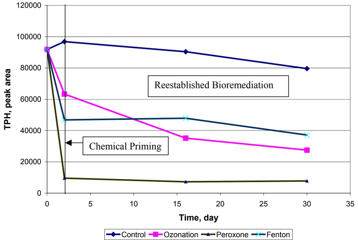
Figure 5.2. HMW-Soil Heavy TPH Results of Chemical Priming and Reestablished Bioremediation
