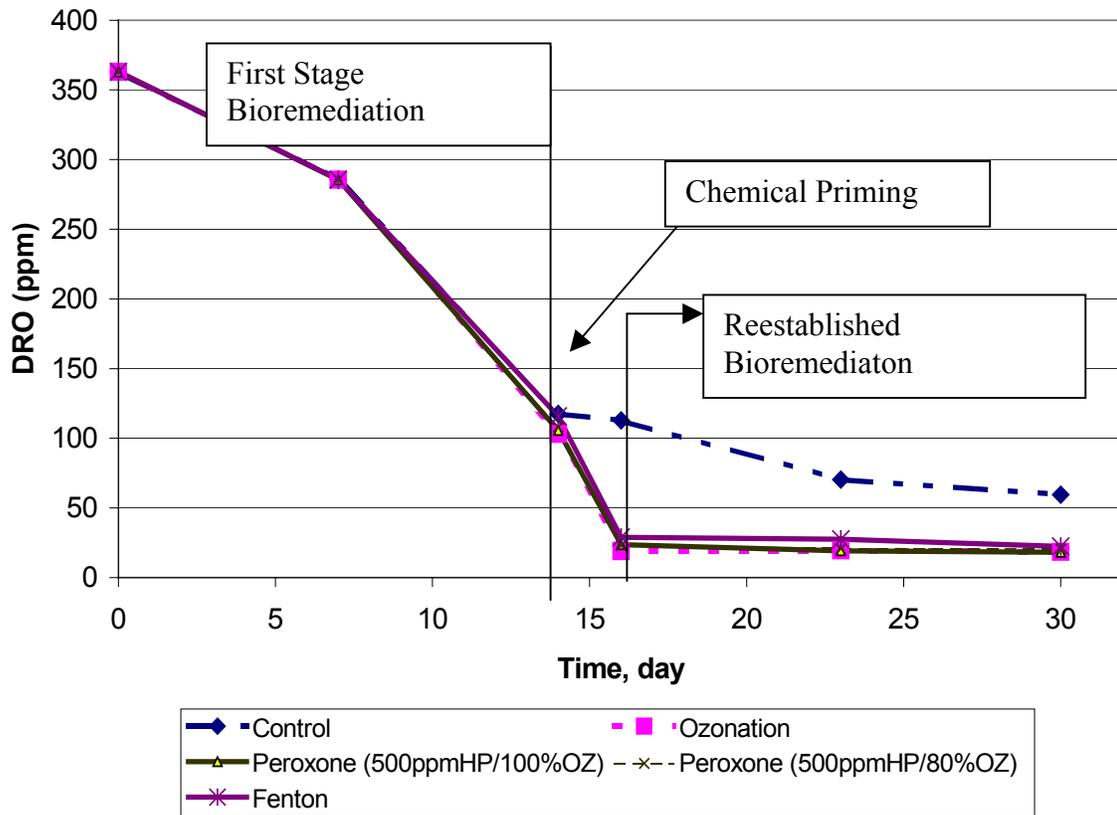
Figure 5.8. BIO/OX/BIO Treatment of the LMW-Soil
