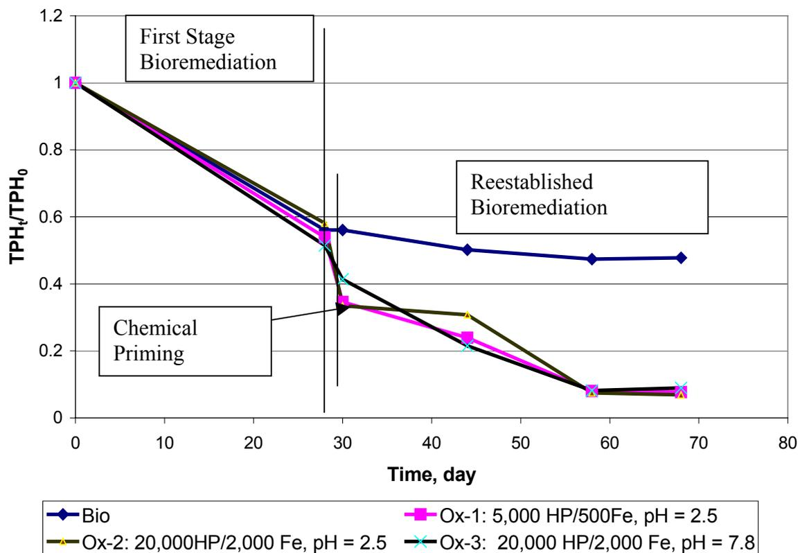
Figure 4.9. Heavy TPH Results of Fenton's Reagent Enhanced Bioremediation for the LMW-Soil
