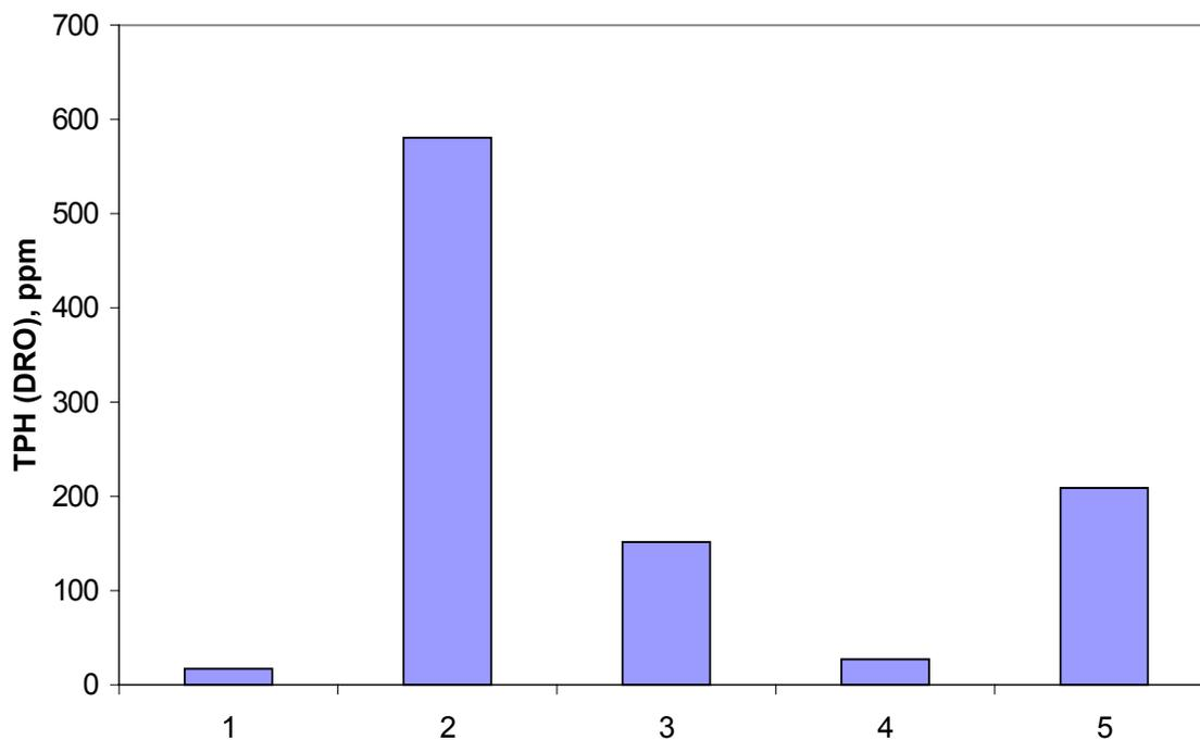
Figure 4.3. Aqueous Phase TPH Results of Slurry Phase Chemical Priming for the HMW-Soil
