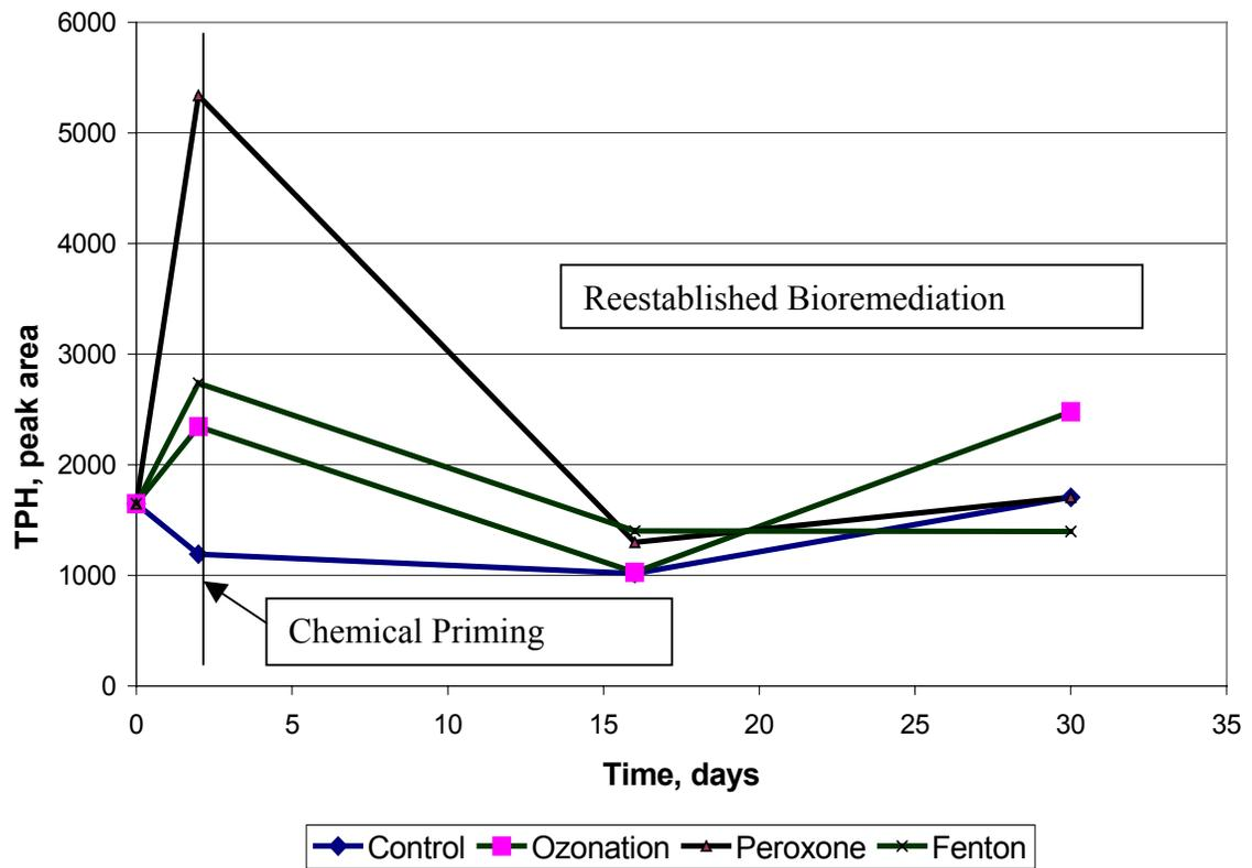
Figure 5.3. HMW-Soil Light TPH Results of Chemical Priming and Reestablished Bioremediation
