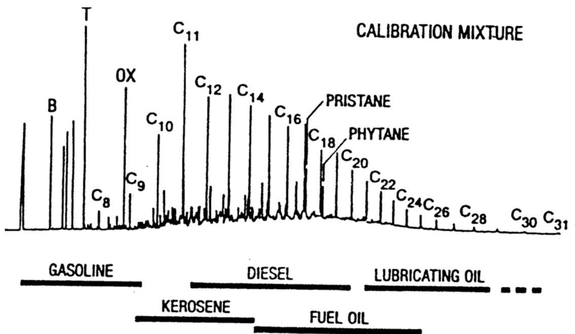
Figure 1.1. Approximate Boiling Ranges for Individual Hydrocarbon Products
