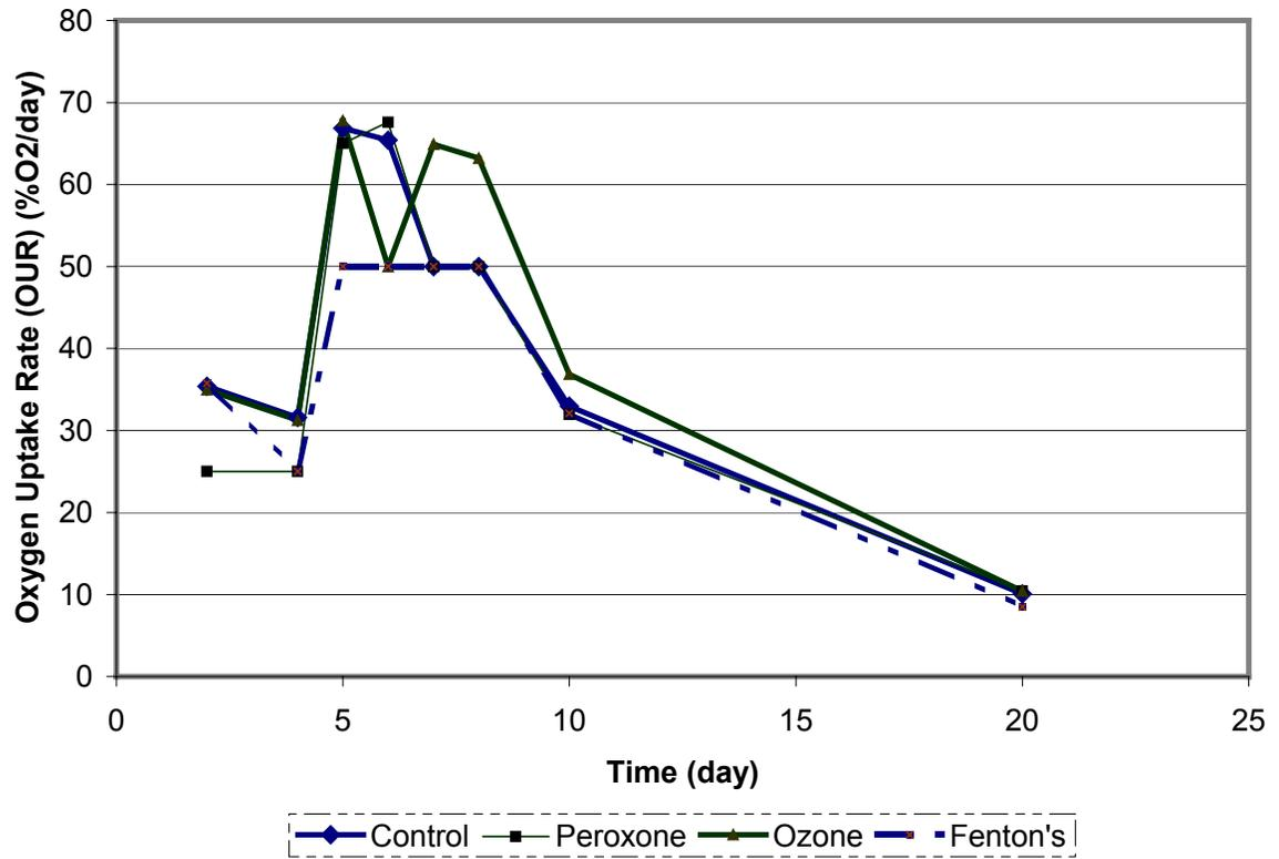
Figure 5.4. O<sub>2</sub> Evolution from Reestablished Bioremediation – HMW-Soil
