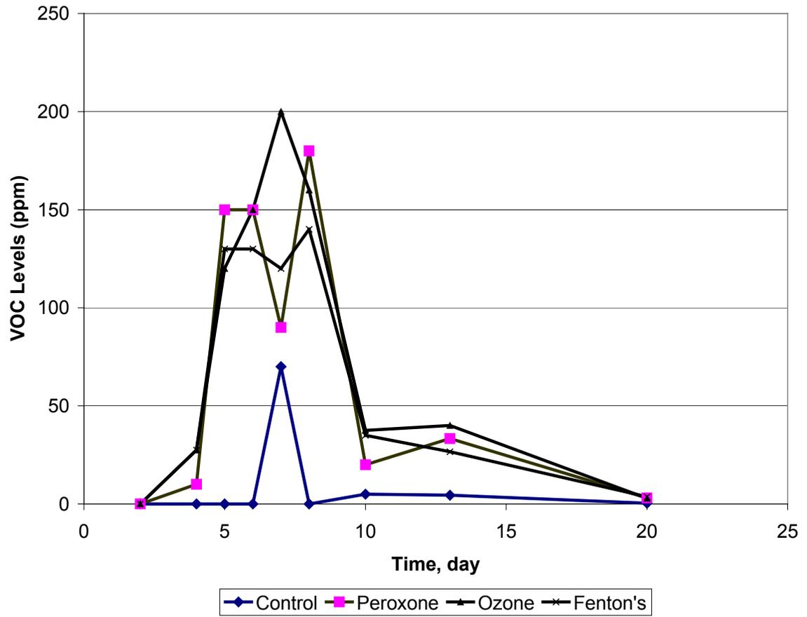
Figure 5.6. Headspace VOC Levels during the Reestablished Bioremediation Stage - HMW-Soil
