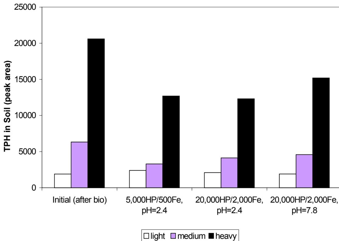
Figure 4.5. Soil Phase TPH Results of Slurry Phase Chemical Priming for the LMW-Soil
