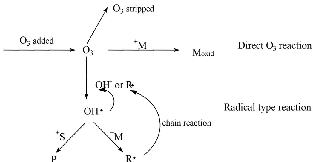
Figure 2.1. Reaction Scheme for Ozone Added to an Aqueous Solution (Hoigne, 1982)
