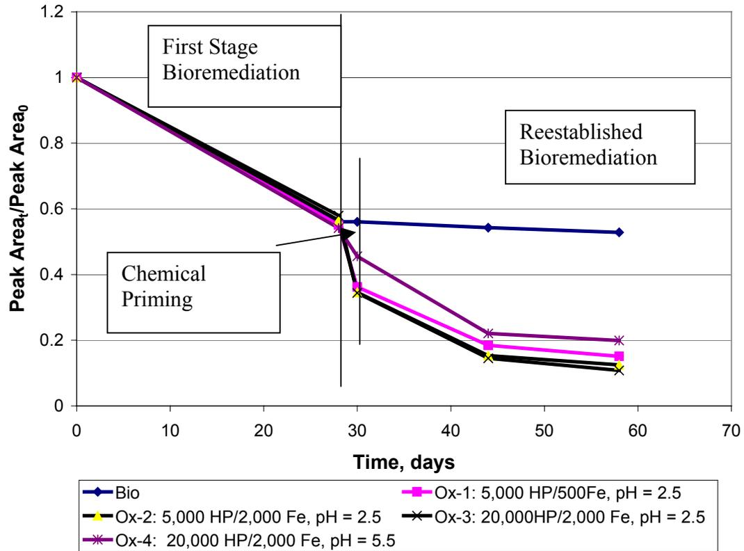
Figure 4.8. Heavy TPH Results of Fenton's Reagent Enhanced Bioremediation for the HMW-Soil
