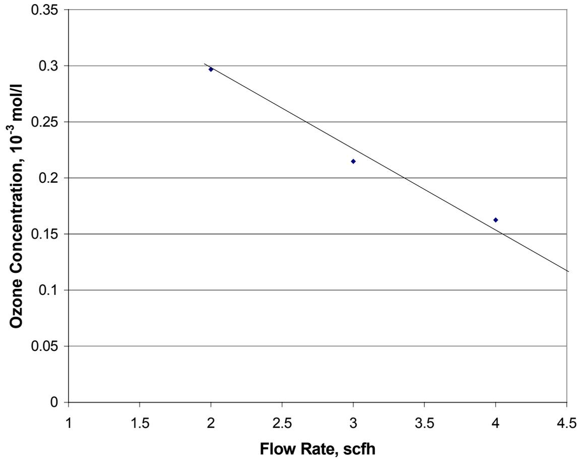
Figure 3.2. Ozone Concentration vs. Flow Rate (Voltage = 112 V)
