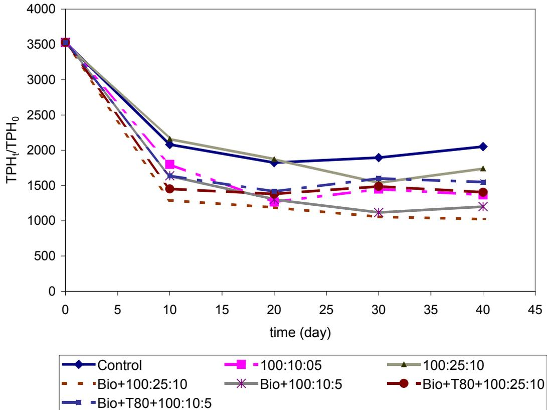
Figure 4.1. LMW-Soil Slurry Phase Initial Bioremediation Results
