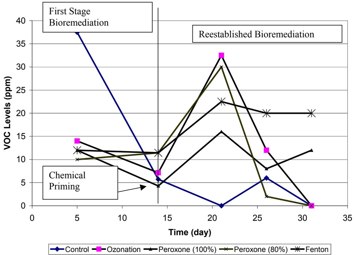
Figure 5.12. Headspace VOC Levels in BIO/OX/BIO Treatment of the LMW-Soil
