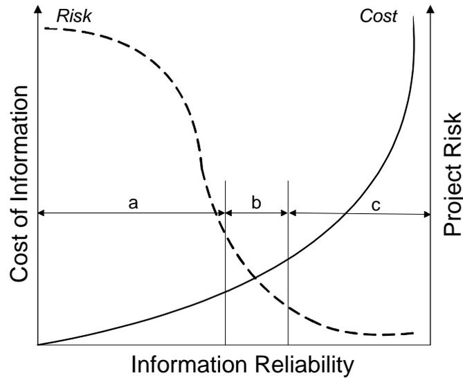
**FIGURE 1 The effect of subsurface utility information on project risks**
