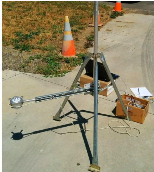
1 2 Figure 1. Albedo measurement system with a dual-pyranometer and DAS.
