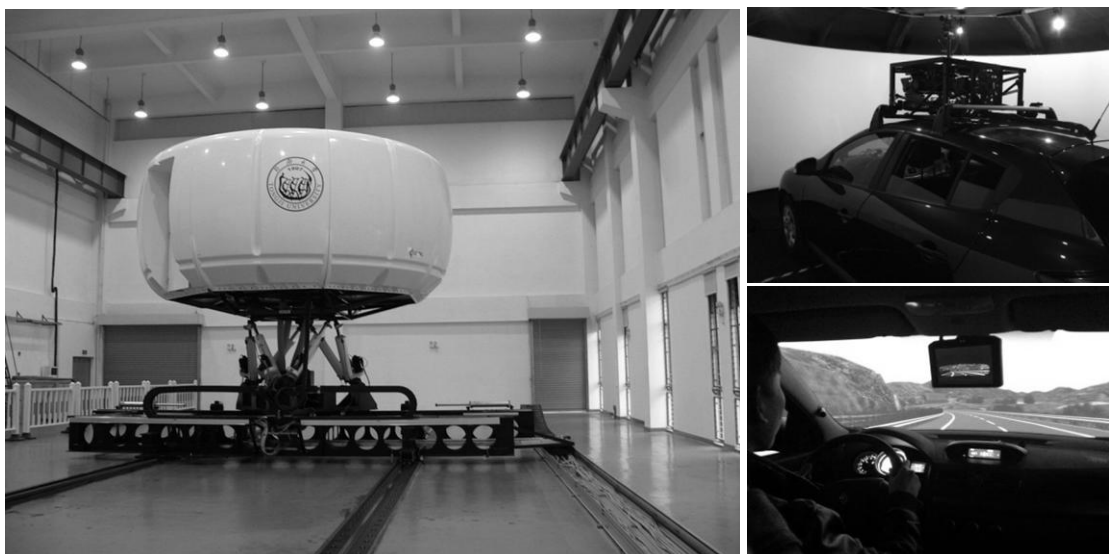
30 FIGURE 1 Tongji advanced driving simulator
