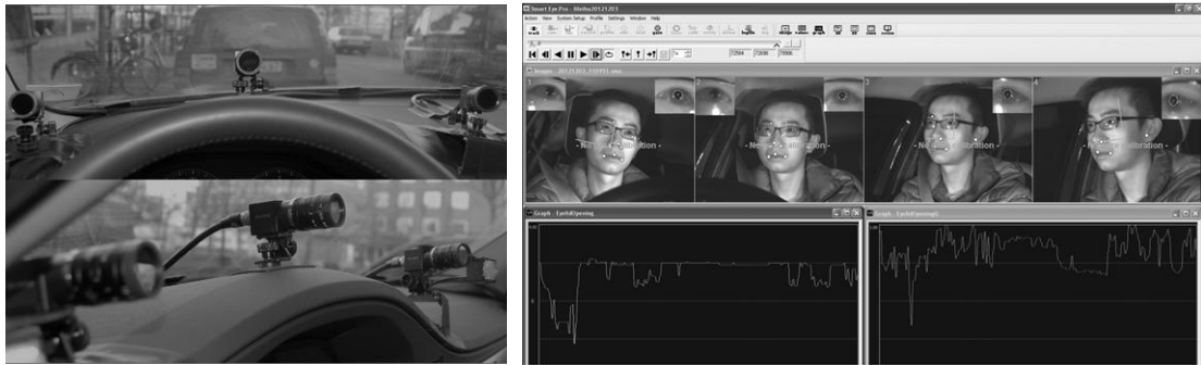
5 6 FIGURE 2 Smarteye® eye tracking system hardware and software interface 7
