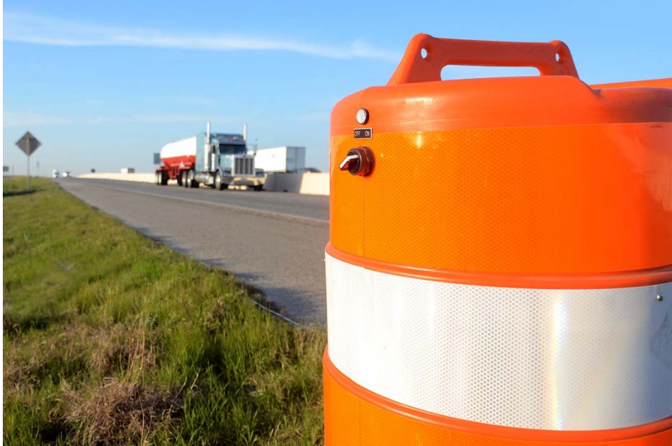
2 (a) iCone™ speed radar sensors housed in a channelizing drum.
