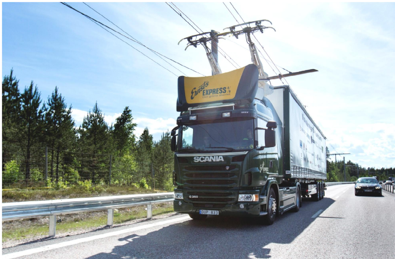
24 FIGURE 2 Hybrid truck in electric operation on public road in Sweden.
