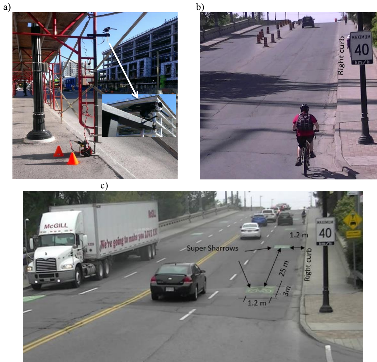
FIGURE 3: Camera position at the site location. (a) video camera set-up. (b) video frame phase 1 (pre-treatment). (c) video frame of phase 4 (post-treatment).
